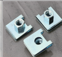
Name: Base nut snap reed nut clip P/N: JX-M6-L23-W20.23-65Mn Material:Steel+65Mn
